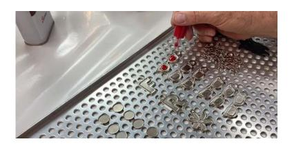
Enamel dosing units, enamelling tables, drying ovens, scales for the correct weighing of the mixture.
